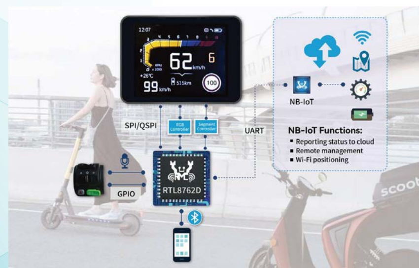
Figure 1 - The Realtek RTL8762DK supports various modes of functionality for e-Bike and e-Scooter dashboards. Image provided courtesy of Realtek.
