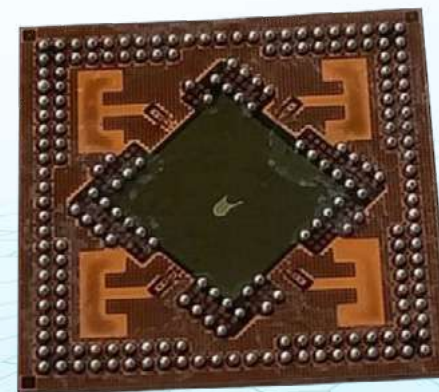
Underside of the AiP with solder ball
