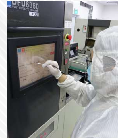
Wafer dicing operation
