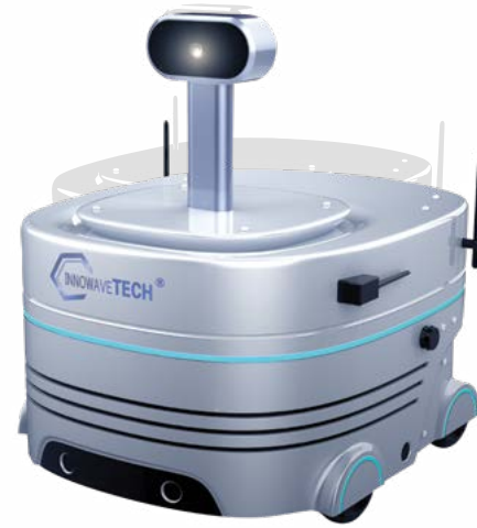
Figure 1 - AGV mounted with optical and thermal cameras to detect water leakage
