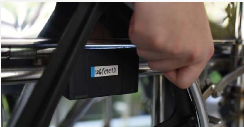
(Photo Credit: Khoo Teck Puat Hospital) Battery-powered wireless tag device installed on 150 wheelchairs at Khoo Teck Puat Hospital, with location information routinely sent to a nearby router beacon for real-time location tracking.
