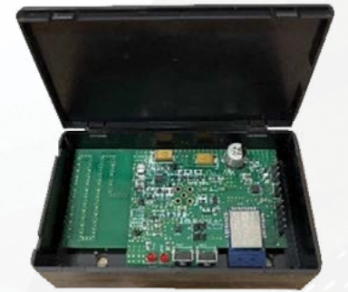
(Photo Credit: A*STAR) Interior of a wireless tag device, which transmits wheelchair location and battery status information to a coordinator via ZigBee wireless technology.
