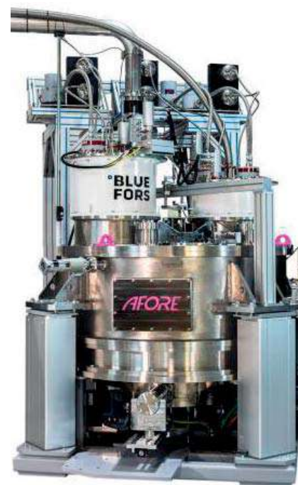
Cryogenic wafer prober, enabling quantum computing
