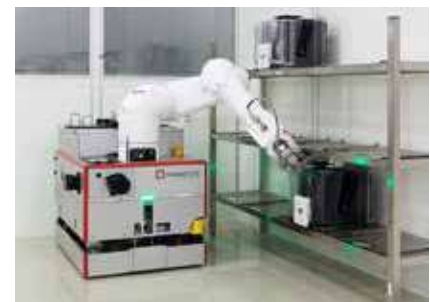
Mobile Robot HERO®FAB 300 handles in different heights from 200 to 1,500mm
