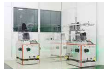
Fully free-moving platform: Ultimate maneuverability thanks omni-directional drive technology
