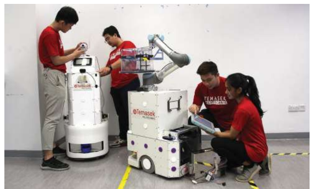
TP AMR integrated with Collaborative Robotic Arm
