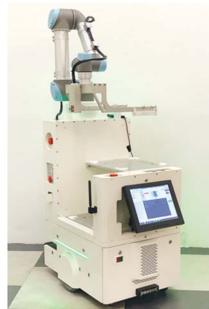
AGV/AMR – Autonomous Mobile Robot with Integrated Robot Arm
