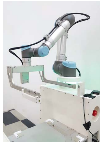
End effector attached to robot arm – designed by CEI
