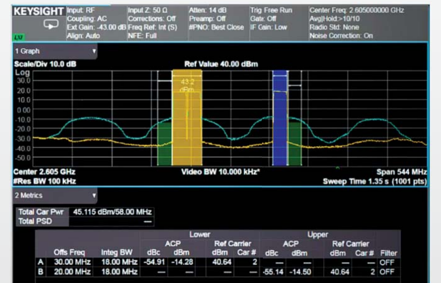
Figure 5: ZCU111 evaluation board based RFSoc setup for 2c LTE20 + 1c LTE with IBW of 160MHz
