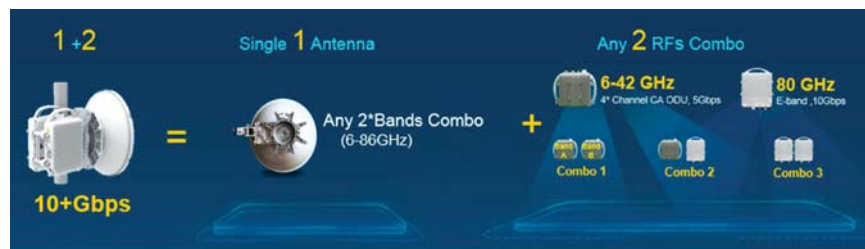
The "1+2" 5G Microwave Architecture
