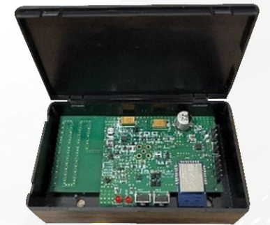
(Photo Credit: A*STAR) Interior of a wireless tag device, which transmits wheelchair location and battery status information to a coordinator via ZigBee wireless technology.
