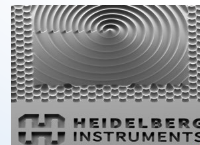
Combined structures: micro lens array (dia 20µm) & Fresnel Vortex Axicon; angles from 22° to 45°, Height 10 µm by Heidelberg Instruments, a member of the LAB14 Group
