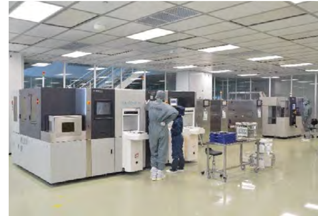
Class 1K cleanroom (size: 276.8m2) at DISCO Hi-Tec Singapore
