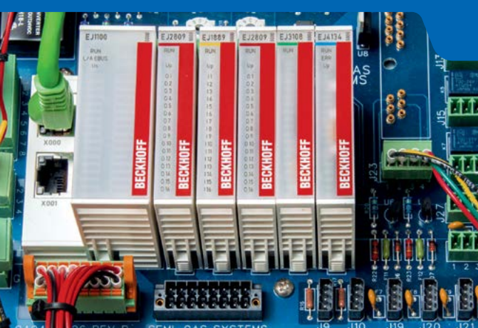
EJ-series EtherCAT plug-in I/O modules fit inside the 8" tall, 10" wide and 12" deep enclosure
