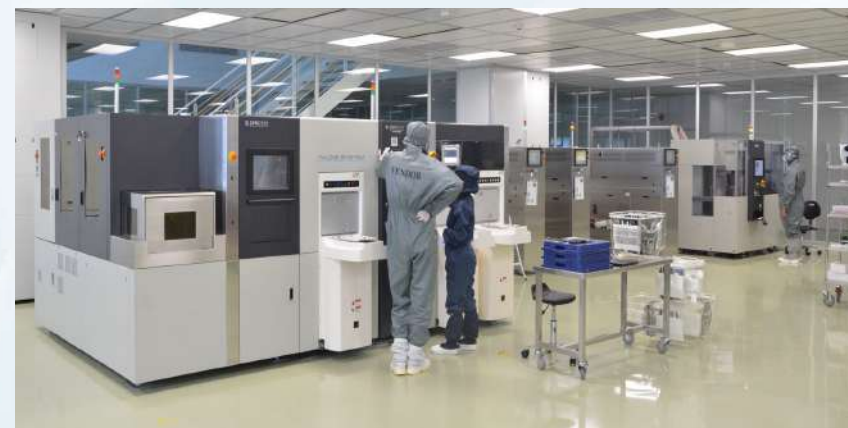
Class 1K cleanroom (size: 276.8m 2 ) at DISCO Hi-Tec Singapore
