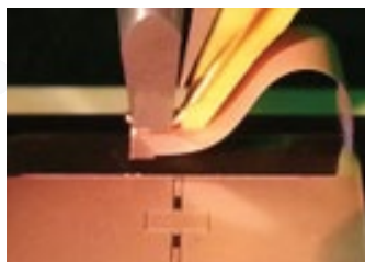
Figure 3: Due to a high stiction force, the bond tool ripped off delaminated surface metallization after the bond tool lifted off from the surface.
